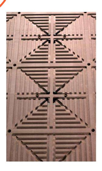
Powerful, partitioned, adjustable vacuum system, adaptable to any type of material and concentrated where needed in the working area. It allows the best fixing during the cutting procedure and the highest energy saving at the same time.
