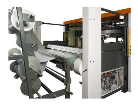
Roll holders of different sizes and capacities useful for processing both single and multilayer sheet materials are available to facilitate the loading operations.
