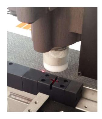
Less wear of the cutting belt thank to knife checking at regular intervals. The monitoring of the knife use is simplified thanks to the machine reporting system.
